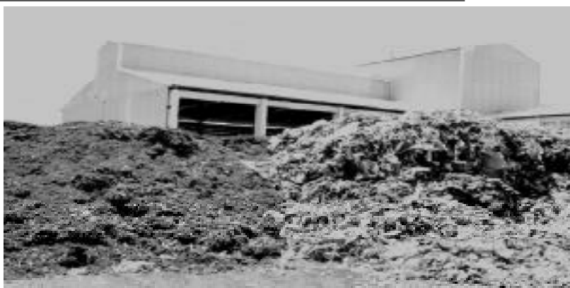
One shift production of Mysore's centralized compost plant; heap of sieved saleable compost on the left, unwanted plastic on the right (larger heap). Highlights the unimagined problem of plastics in waste.
